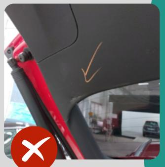
• Cracks and larger nicks (for example, caused by load or stains from chemicals) or damage to the luggage compartment cover are unacceptable (K4-K5).
