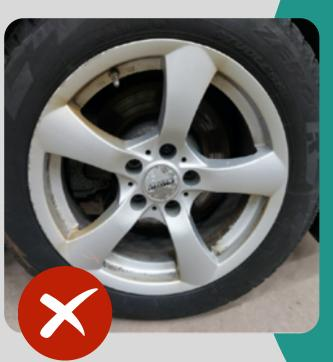
Damage from collision from curb stone is unacceptable (K4-K5).
