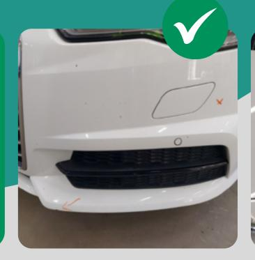
Minor stone chips up to 10 mm without rust are acceptable (K1-K3).
