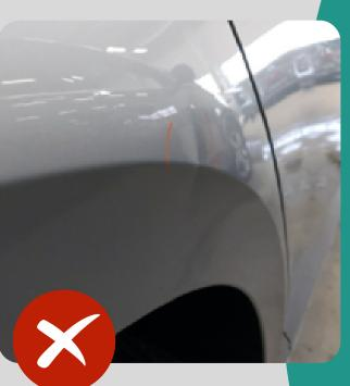
Larger deformations with a diameter of more than 25 mm are unacceptable (K4-K5).
