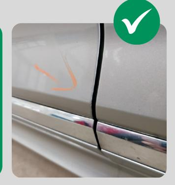
• A maximum length of 20 mm is acceptable, without start of corrosion or deformation of edge (K1-K3).
