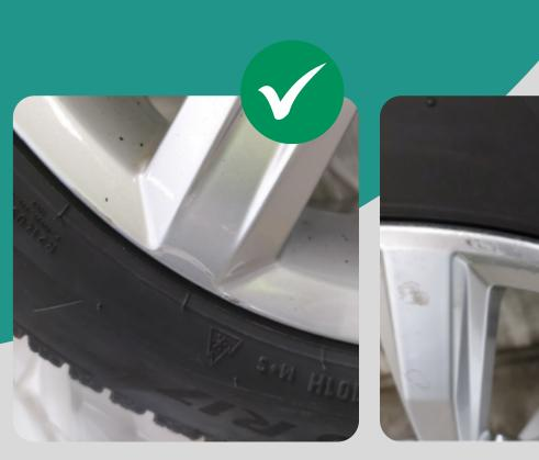
The acceptable length of a scratch is 50 mm - maximum of 2 per wheel (K1-K3).
