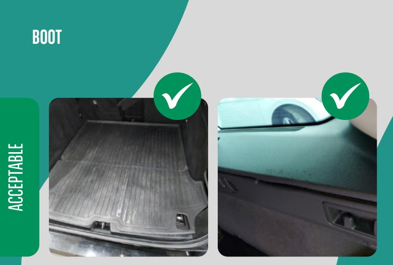
• Only surface scratches without larger nicks are acceptable (K1-K3). If the vehicle has a boot partition, this must be returned along with the vehicle.
