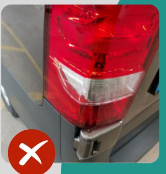
• Larger scratches, cracks and stone chips are not acceptable (K4-K5).
