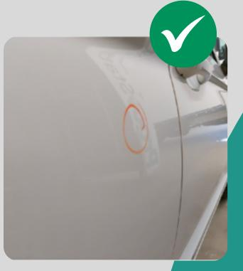
Minor deformations with a diameter less than 25 mm, without damages to paintwork and start of corrosion are acceptable (K1-K3).
