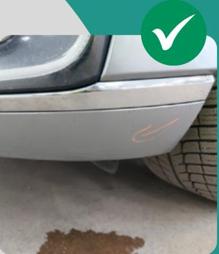
• A scratch, that can be removed by polishing, is acceptable (K1-K3).
