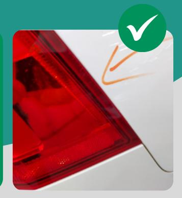
Minor scratches having no influence on functionality and aesthetic appearance or cracks are acceptable (K1-K3).
